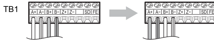
Figure 11: A Channel and B Channel Wire Switching
