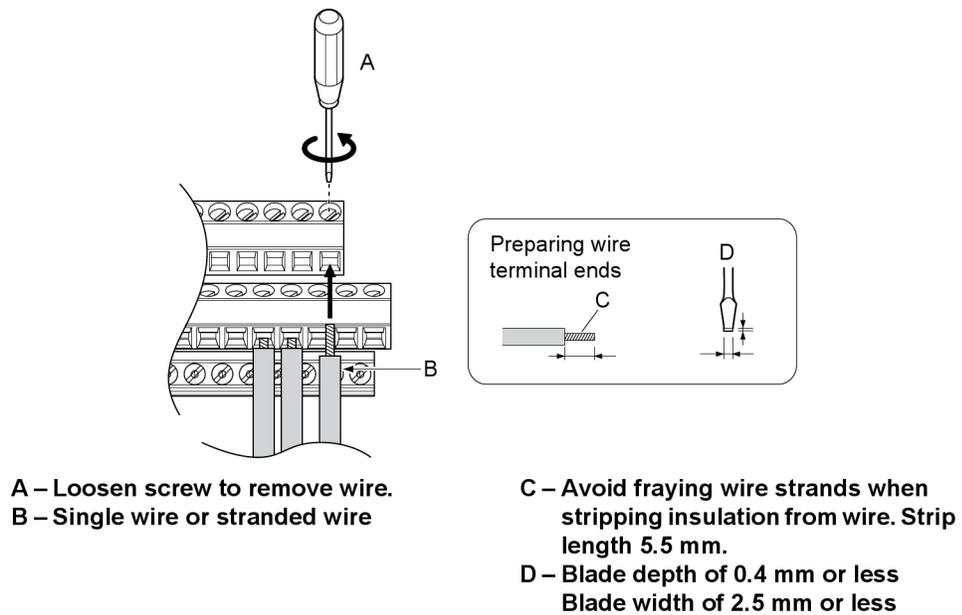
**Figure 3: Terminal Board Wiring Guide**
