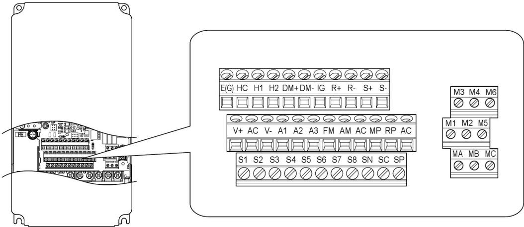
Figure 2: Control Circuit Terminal Arrangement
