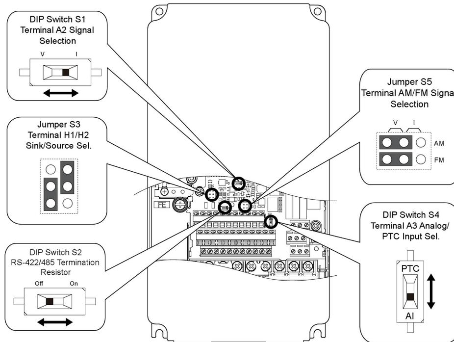
**Figure 4: Locations of Jumpers and Switches on the Terminal Board**
