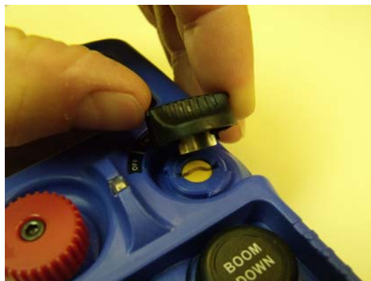
Figure 8: Machine Stop Switch and OFF-ON-START rotary
