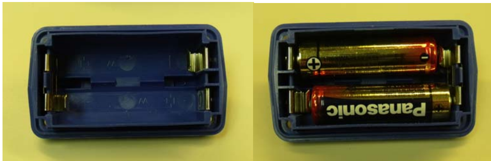
Figure 5: Separated Alkaline Battery Pack
