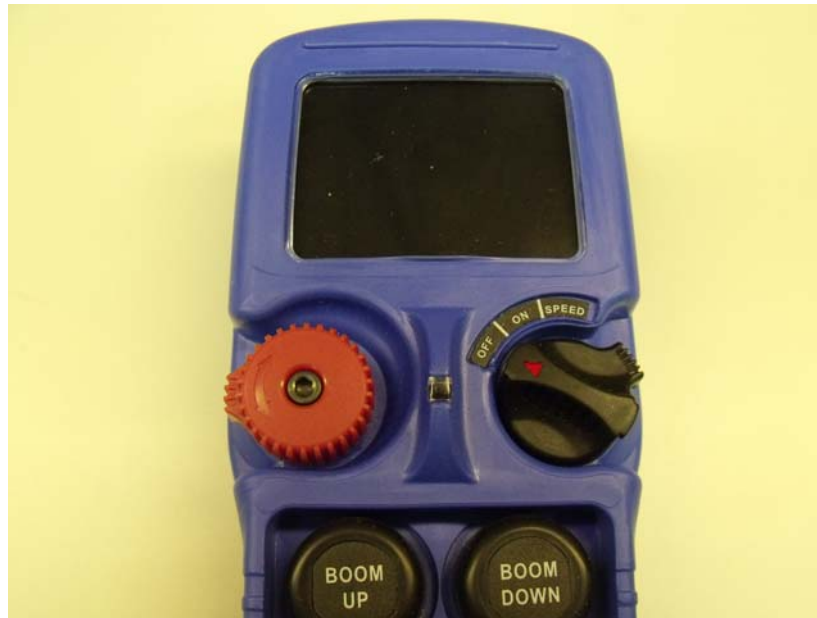
Figure 7: Machine Stop Switch and OFF-ON-START/SPEED rotary
