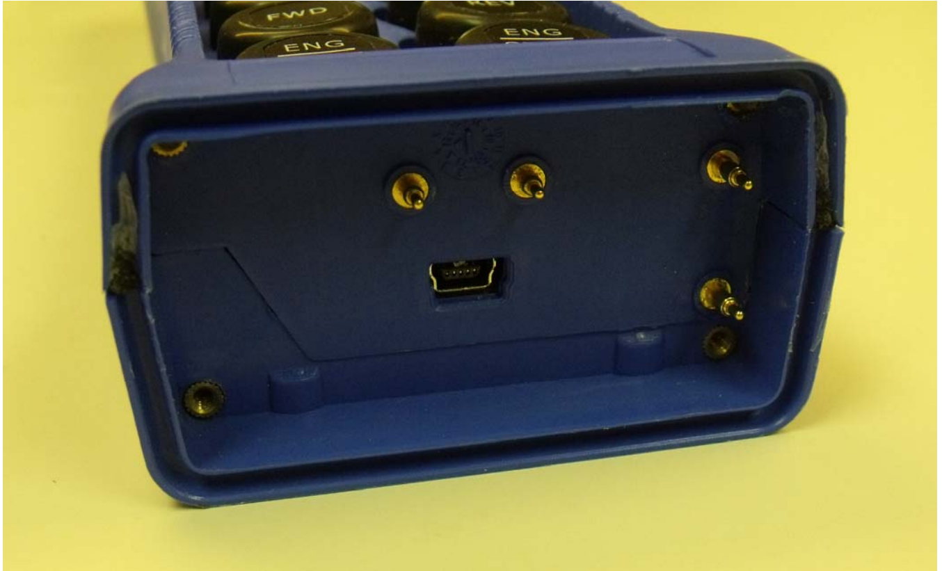
Figure 10: USB mini-B receptacle as viewed through the battery compartment
