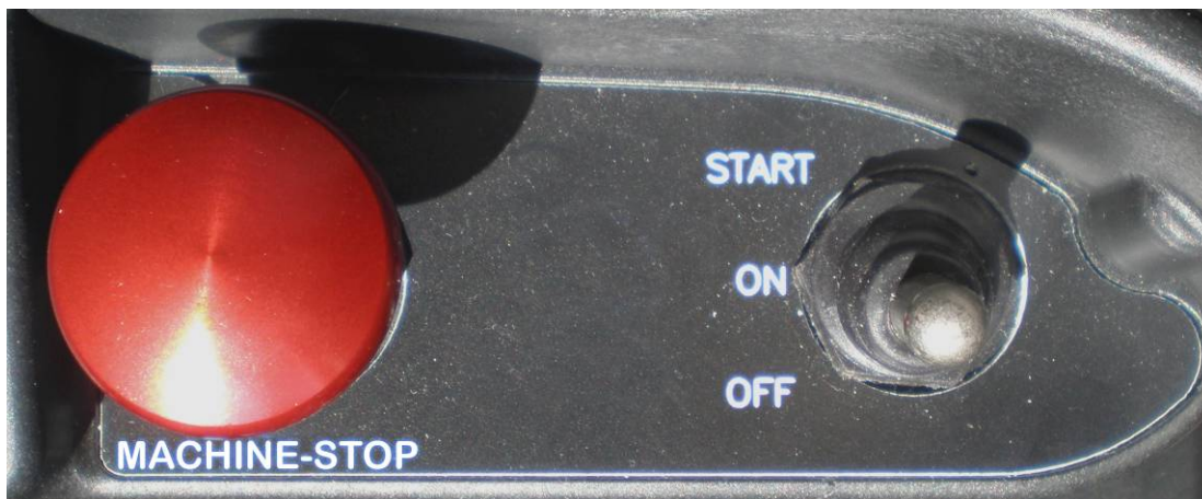
Figure 10: Machine Stop Switch and OFF-ON-START toggle
