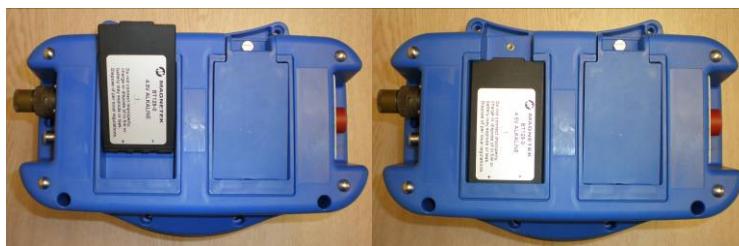
Figure 4: Installation of Battery Pack into XLTX transmitter
