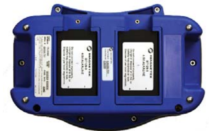
Main battery and spare battery packs
