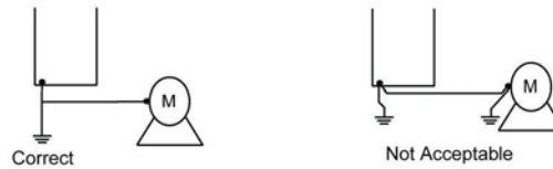
Figure 3-3: Grounding the Motor
