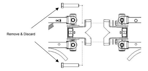
3 – Re-assemble mounting bracket assembly with the UC-EXT-200 Extension Bracket as illustrated below. Do not tighten hardware until collector assembly is properly located on mounting post.
