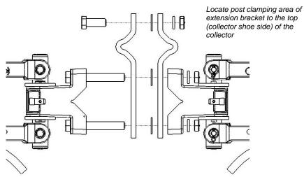
4 – When collector is properly aligned with the conductor bar, tighten hardware. Tighten each bolt until the collector is firmly in place on mounting post (30 to 38 lb.ft.). *Note: The size of the mounting posts may vary – if the extension bracket is not firmly gripping the mounting post after the bolts are tightened, remove the bolt from above the post, remove the spacer washer, replace the bolt and re-tighten.*
