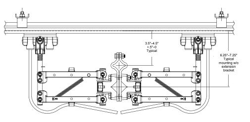
UC Type Collector Mounting With Extension Bracket
