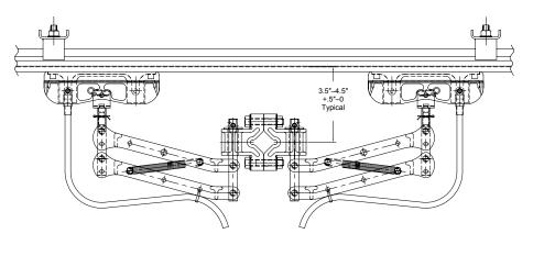
PC Type Collector Mounting Configuration
