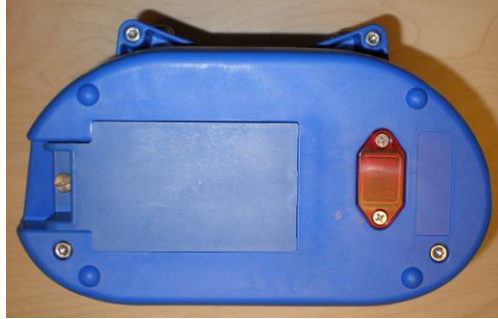
Figure 5: Installation of Battery Cover
