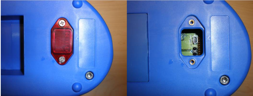
Figure 7: USB/IR Cover Location and Cover Removal
