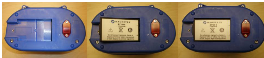
Figure 4: Installation of Battery Pack into MLTX2 transmitter
