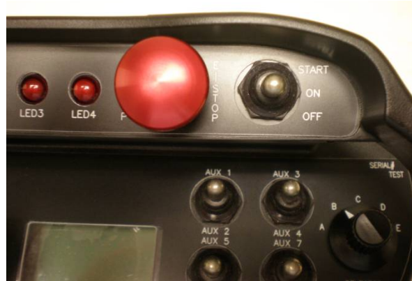
Figure 9: Machine Stop Switch and OFF-ON-START toggle
