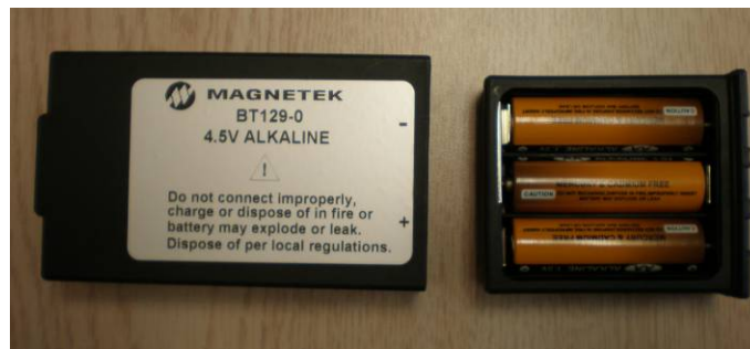
Figure 3: Separated Alkaline Battery Pack
