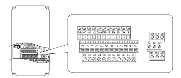
Figure 2: Control Circuit Terminal Arrangement
