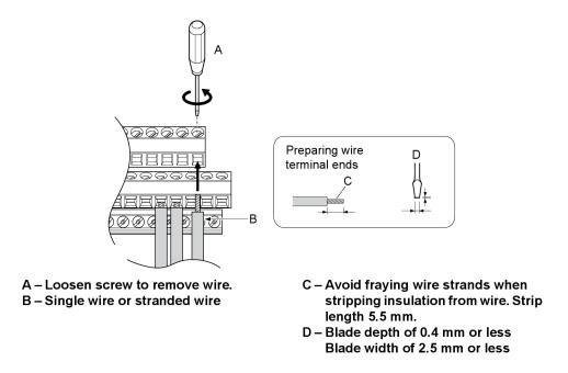
Figure 3: Terminal Board Wiring Guide
