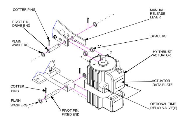
**9.2.(f):** Secure or support the actuator before attempting to remove the pivot pins.
