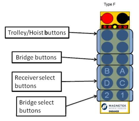
f. In case of an emergency, pressing down on the red emergency stop button will immediately disconnect the receiver mainline (Status LED blinks red). To reset the emergency stop button just rotate the red button either clockwise or counter-clockwise; it will pop up. When the green light appears, rotate the power key to "Start" position to resume operation (depends on JP3 setting on page 24).
