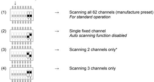
\*If the first 6 dip-switch positions on the receiving module is set to Ch.01 ("000000" or "000001"), when set to 2-channel scanning (type-3 above), then the receiver will only scan Ch.01 and Ch.02.
