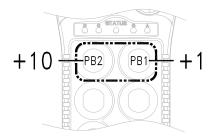
Examples: Press PB2 two times and then PB1 four times will give you channel 24. Press PB1 nine times with give you channel 09.
