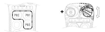
b. Select a new channel by pressing PB1 and PB2 on the transmitter. Press PB1 to increment the units (+1) and PB2 to increment the tens (+10).
