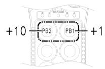
Examples: Pressing PB2 two times and then PB1 four times will give you channel 24. Pressing PB1 nine times with give you channel 09.
