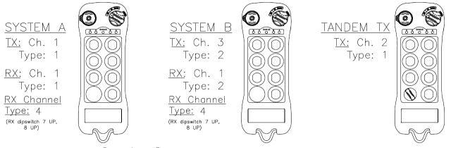
NOTE: "PITCH/CATCH" FEATURE SHOULD BE DISABLED FOR THIS APPLICATION. TO DISABLE, SET RECEIVER DIPSWITCH 4 (FOR FLEX 8EX) OR 6 (FOR FLEX 12EX) TO THE FOLLOWING: DIP 7 UP, ALL OTHERS DOWN (00000010)
