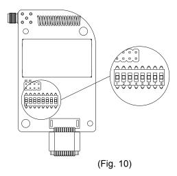
Even though the Flex system is equipped with an automatic channel scanning receiver, the user can also set the receiver channel manually. Please refer to page 24 on how the automatic channel scanning receiver works.
