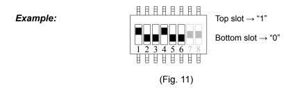
The above dip-switch setting "1 0 0 1 0 0" corresponds to "channel 36" in the system channels table on page 29.
